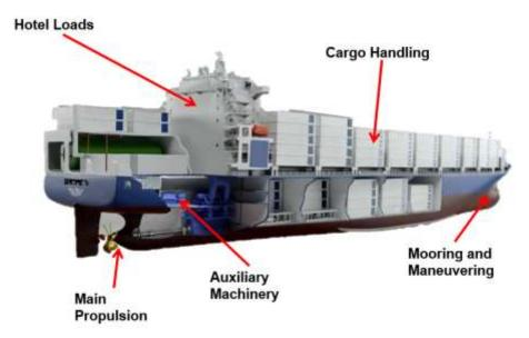
Figure A.1. Common energy consumers on a ship.
